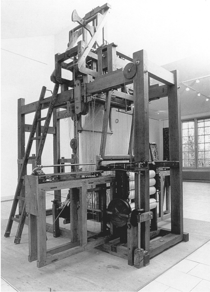
FIGURE 10. Vaucanson's automatic loom. From Claudette Balpe, "Vaucanson, mécanicien et montreur d'automates," La Revue , no. 20 (Sept. 1997): 36.
